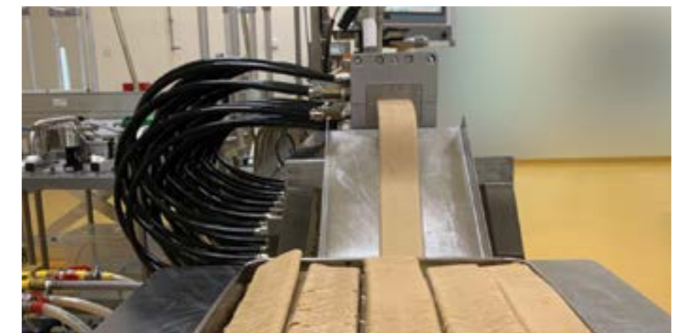
The extruder that texturises plant-based proteins into viable meat alternatives. A similar extruder will be available at the upcoming FoodPlant.
