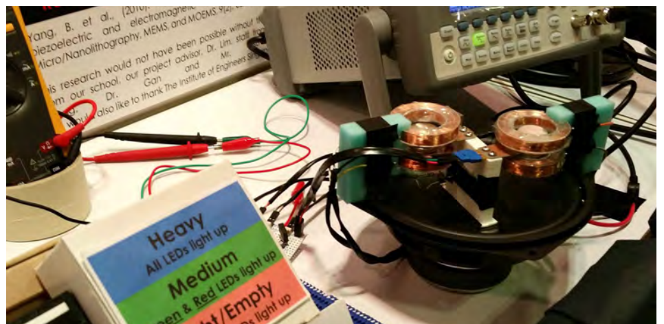
The prototype harvests vibrational energy and uses this to power a signalling system for MRTs.
