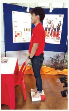
Users are required to step on the device, while holding on to a weight-cross bar such as the back rest of a chair.
